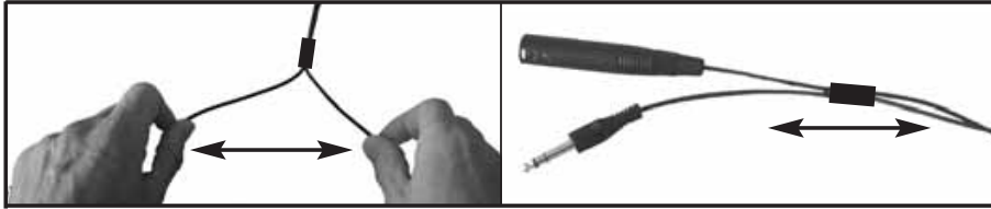
Fig. 2: Separating microphone and headphone cables.
